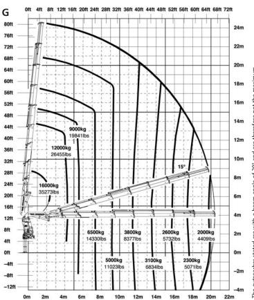
The outreaches stated are with a boom angle of  $20^\circ$  and are therefore not the maximum.
